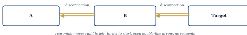
Figure 21.1. Forward synthesis reasons start-to-target with ordinary arrows carrying reagents; retrosynthesis reasons target-to-start with an open double-line arrow and no reagents — it records a disconnection, not a reaction.
